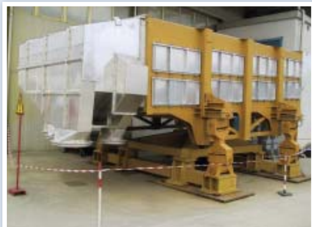
Wood-chip sorting screen mounted on 8 pcs. AK 100-4 suspensions
