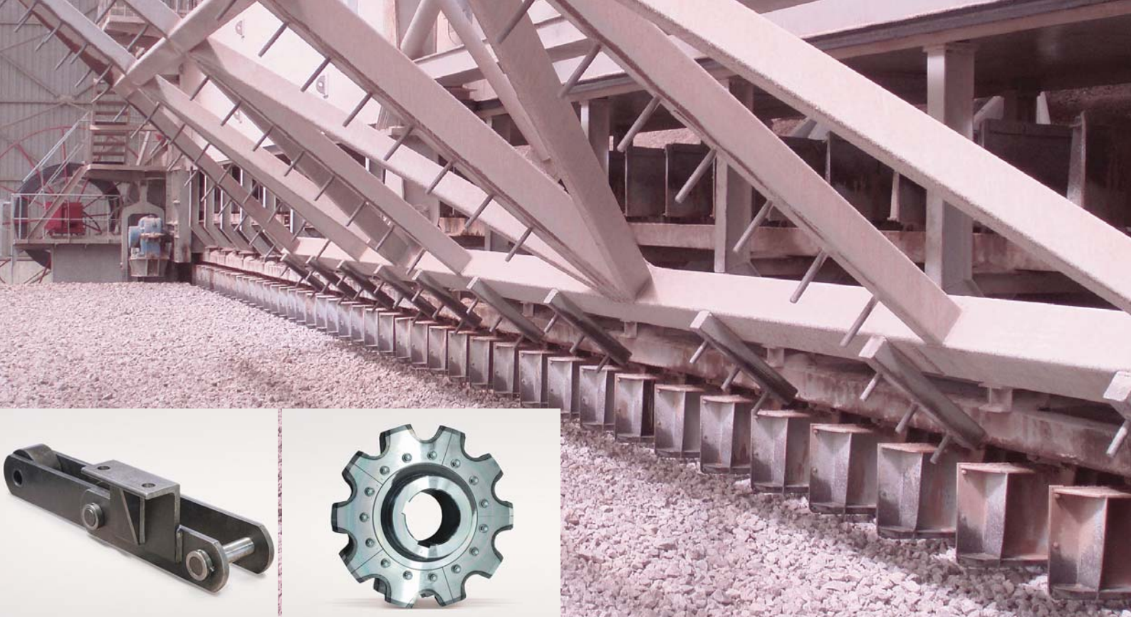
Twin Stranded Bushed Chain with Plain Roller and Welded Attachment Bracket
