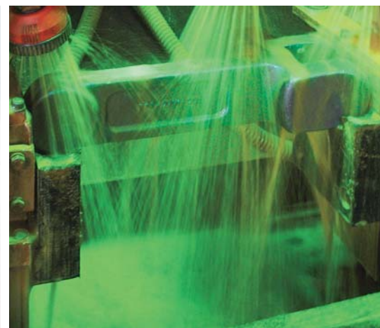
Magnetic Crack Testing of Forged Link
